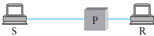
Figure 8.23 Simple internet, with source S sending message to receiver R through proxy P.
