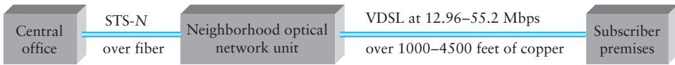
Figure 2.4 VDSL connects the subscriber to the optical network that reaches the neighborhood.
